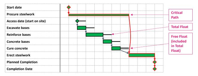
The 5 weeks of civil works activities are seen to have a week of float, generated by the elongated (7 week) procurement period for the steelwork. That may well be realistic, but if there is a delay to the civil activities (for example, a delay in access, or a prolonged excavation due to ground conditions) which causes a week's delay, the presence of "float" means it may not generate any claim for EOT (though of course, a claim for the direct costs would still be possible).
