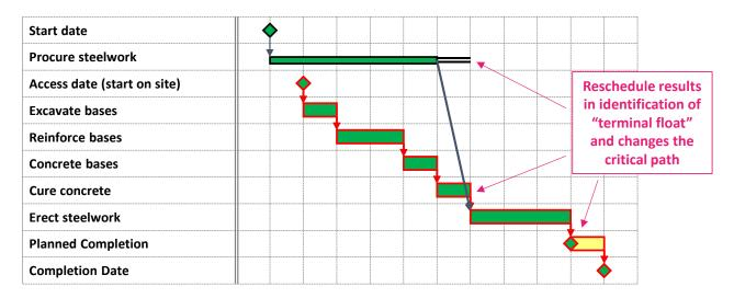
If the programme were adjusted in this way, then any delay in the progress to the physical works will demonstrate a "critical delay" to "Planned Completion" (and thus a claim for time). However, if the Contractor suffers his own delay, he still has the opportunity to "absorb it" (using the terminal float).
